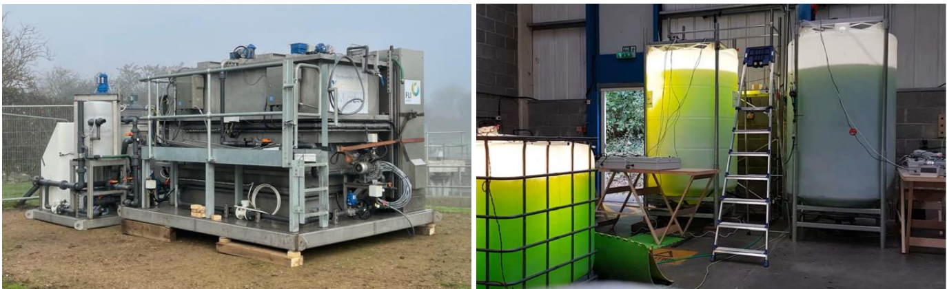
Figure 90 - Proposed nitrogen removal technologies: Microvi (L) and iPhyc (R)
