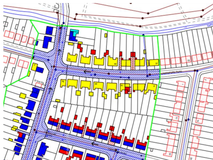
Figure 79 - Impermeable area connectivity results
