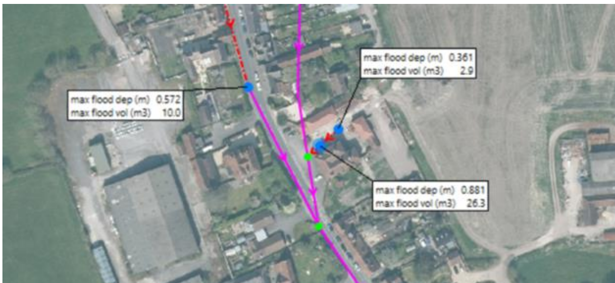
Figure 78 - Example of model predictions plan view and long section
