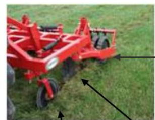
Grassland subsoiler used in West Dorset. Lifted area on left, unlifted area on right. Photo credit: J Franklin.
