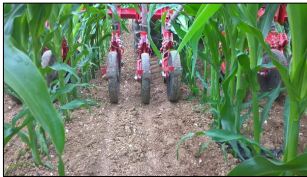
Figure 3: An undersowing drill establishing grass between the rows. Photo source: Wessex Water
