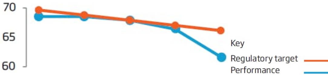
Figure 3.23 Wessex Water leakage volumes (MI/d)
