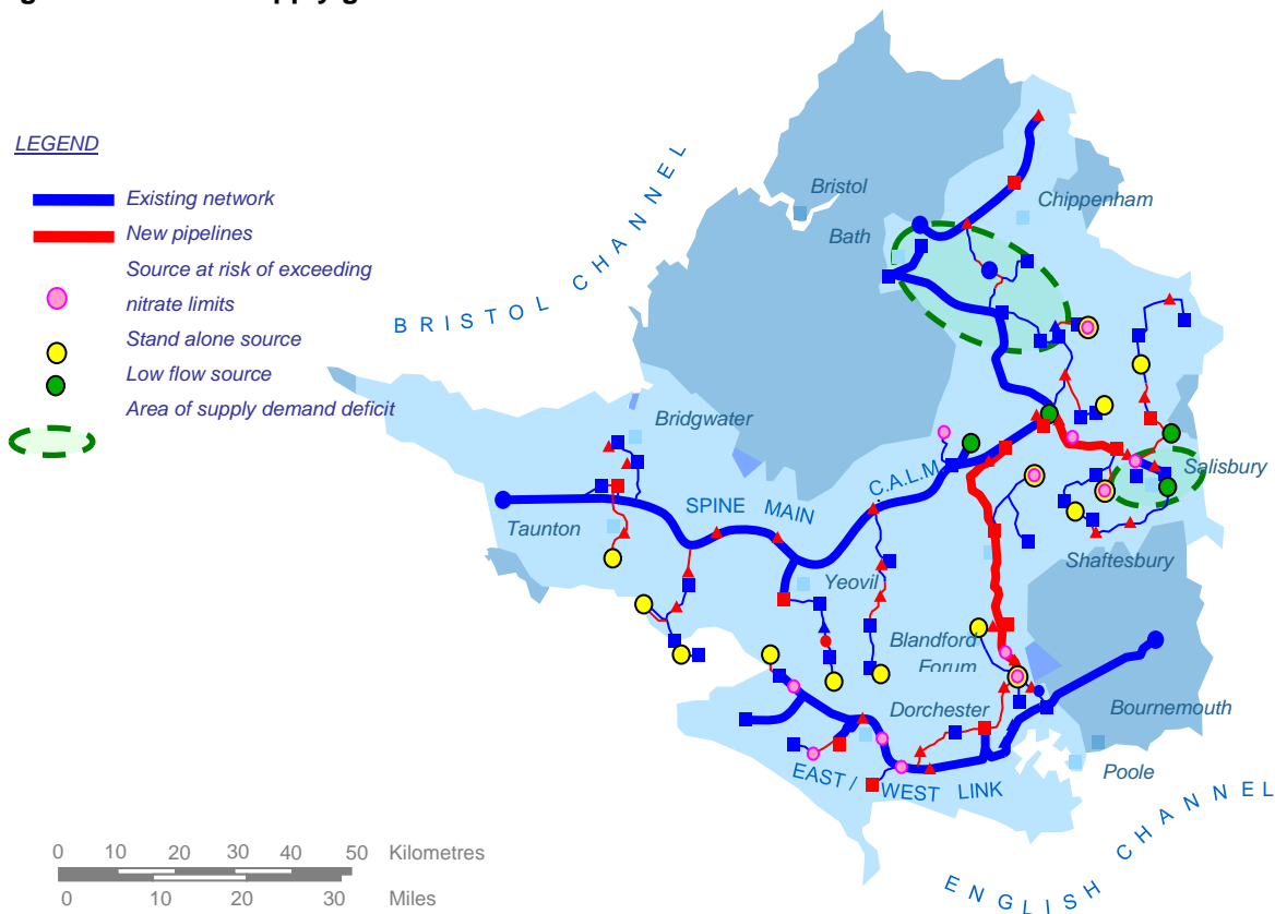
Figure 8-3: Water supply grid
